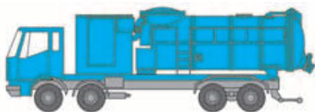
Vacuum loader mounted on truck or trailer, 55 to 350 kW, truck engine or separate diesel engine
