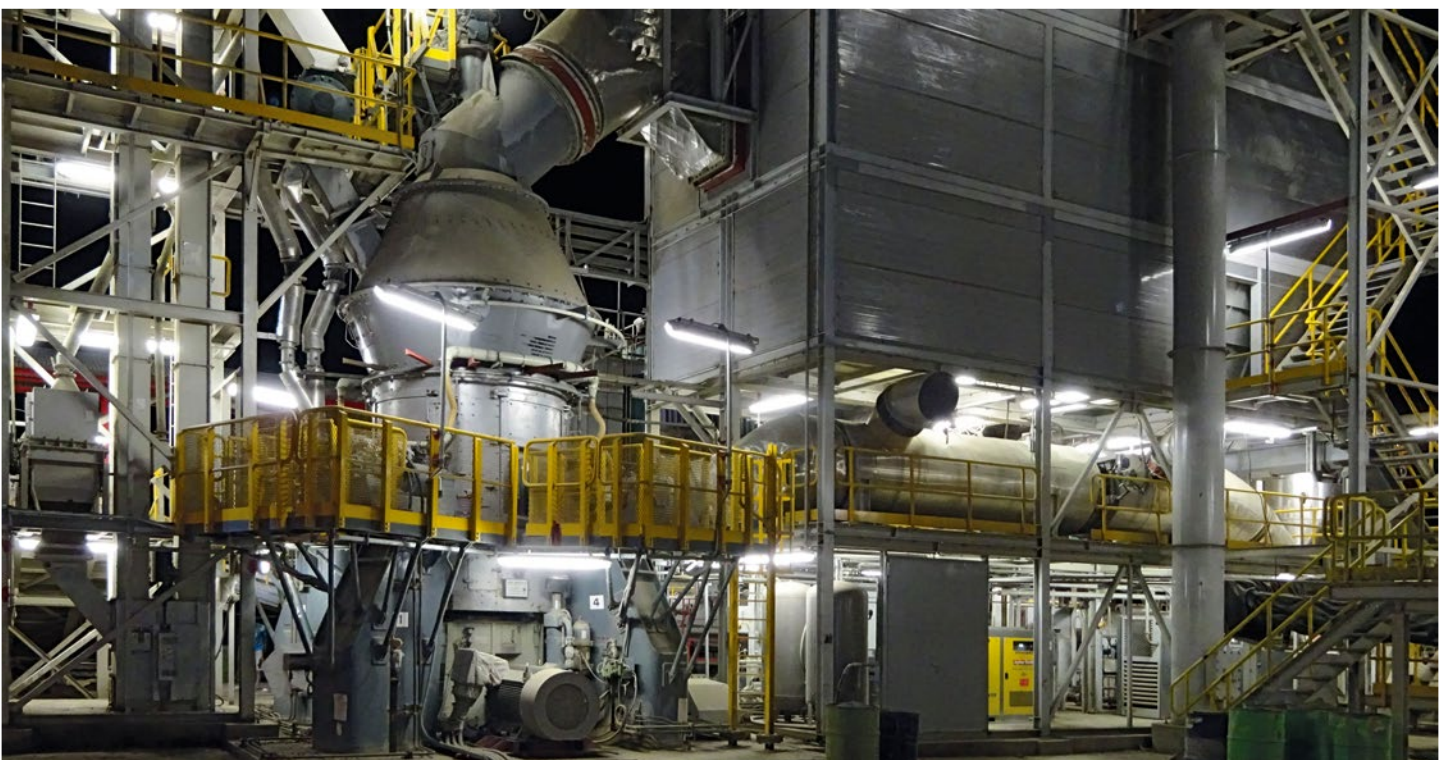
The world's first modular system with a vertical cement mill operating in Africa
